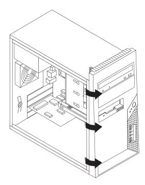
Figure 7. Removing the front bezel
